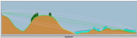
Fig. 5 TV repeater to WA2YUN -- this is an example of an obstructed, short, 1 mile path in which a signal can still be received via diffraction. Pr = -85.9 dBm (predicted) & -81 dBm (measured) +4.9 dB difference
