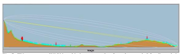
Fig. 7 TV repeater to W0QN -- this is an example of an obstructed, 8.2 mile path in which the received signal is within  $\pm 3 dB$  of receiver sensitivity threshold. This is indicated by the direct rays being plotted in yellow. Pr = -89.3dBm (predicted) & -92dBm (measured) -2.7dB difference
