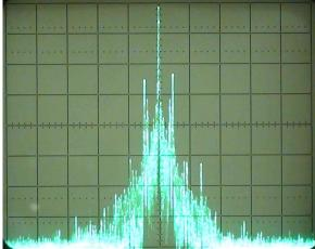
Fig. 2 Spectrum of a typical, commercially available, ham, 70 cm, AM-TV transmitter. (10 MHz/div & 10 dB/div)
