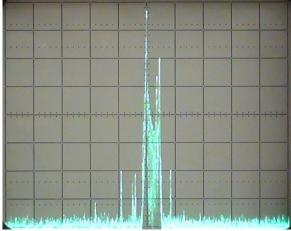
Fig. 3 Spectrum of KH6HTV VIDEO model 70-4, NTSC, VUSB-TV, transmitter (10 MHz/div & 10 dB/div)
