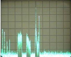
Fig. 1 Typical over the air broadcast spectrum from 150 MHz to 250 MHz The signal in the center is a local, Boulder, channel 11, NTSC analog TV station. Also seen are DTV stations on channels 7 and 9 from Denver. (10 MHz/div & 10 dB/div).
