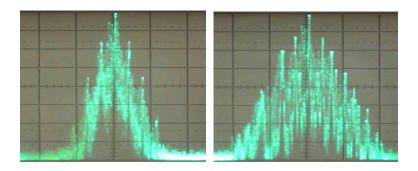
Fig. 3 Spectrum plots of a 4 MHz deviation, FM TV transmitter with pre-emphasis and running with normal, "live", video modulation. 10 dB/div & 10 MHz/div. (left) no subcarriers (right) with stereo sound sub-carriers at 5.8 & 6.2 MHz
