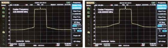
Fig.1 DVB-T, 6 MHz BW Spectrums. Left is modulator output at -3dBm. Right is DVB-T Transmitter output at +30dBm. 10dB/div & 3MHz/div.
