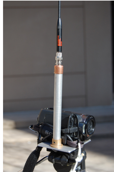
Fig. 3 The Sony hi-def. camcorder and 70 cm, whip antenna, both mounted on a tripod.
