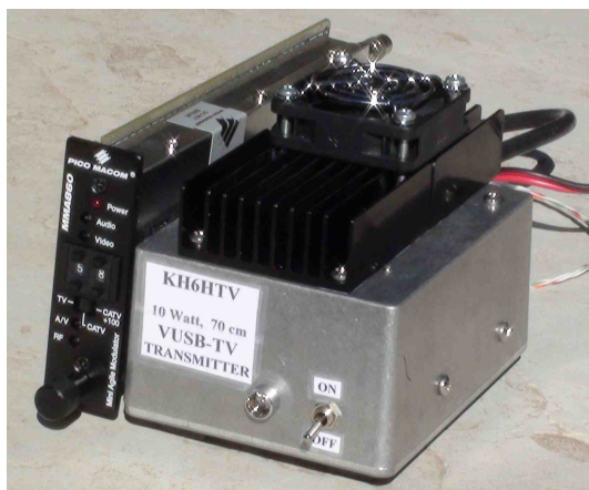
Fig. 4 KH6HTV, 10 Watt, 70 cm, synthesized, NTSC, analog, VUSB-TV transmitter
