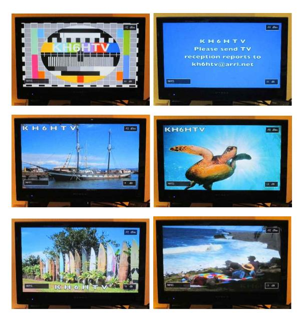
Fig. 5 Various images received by N0YE from KH6HTV. Composite video from prerecorded DVD slide show. Note: upper right hand corner displayed the received signal strength in dBm (no pre-amp). The lower right hand corner displays the S/N in dB.
