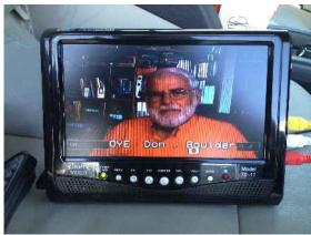
Fig. 2 N0YE's live, 70cm, DVB-T transmission from Boulder as received by KH6HTV in his automobile at the Mead AT&T microwave site on I-25. 24 mile distance, 19dB receive margin.
