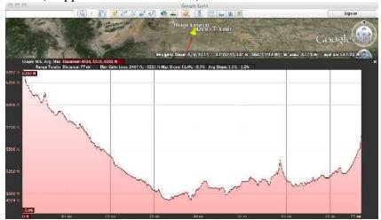
Fig. 4 RF path profile from Cheyenne, Wyoming to N0YE's QTH in Boulder, Colorado. Note: this does not include corrections for the curvature of the earth.
