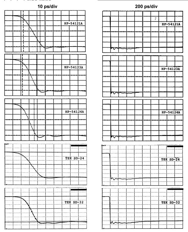
Figure 1: Picosecond Domain Transient Step Responses of HP and TEK Wideband Sampling Heads Input was 13.1 ps falltime step from PSPL 4015B Pulse Generator. Horizontal = 10 ps/div (left) and 200 ps/div (right). Vertical = 50 mV/div. Samplers tested from top to bottom are: HP-54121A (20 GHz), HP-54123A (34 GHz), HP-54124A (50 GHz), TEK SD-24 (20 GHz) and TEK SD-32 (50 GHz).
