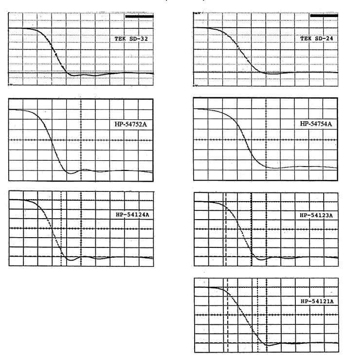
Figure 1: Risetime Performance of Various HP and TEK Digital Sampling Oscilloscopes Input was -300 mV, 13.1 ps Falltime Pulse from PSPL 4015B Pulse Generator. Vertical = 50 mV/div. Horizontal = 10 ps/div.
