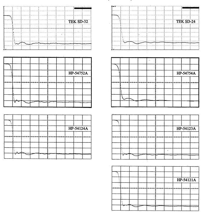
Figure 2: Measurements of PSPL Model 4015B, -300 mV, 13 ps Step Pulse by Various TEK and HP Digital Sampling Oscilloscopes
