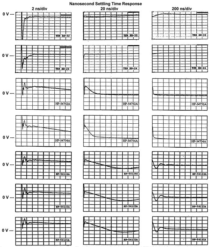
Figure 3: Nanosecond Domain Settling Time Response of Various HP and TEK Digital Sampling Oscilloscopes Input was 420 ps falltime step pulse from 500 mV to 0 Volts from PSPL 6110D Reference Flat Pulse Generator. The reference pulse settles flat to 0 Volts baseline to within 0.1% in less than 5 ns. Vertical = 0.4%/div (2 mV/div). Horizontal scales are 2 ns/div, 20 ns/div and 200 ns/div.
