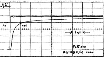
Figure 4: Step Response of a Long Coaxial Cable Showing the Classical Skin-effect "Dribble-up"
