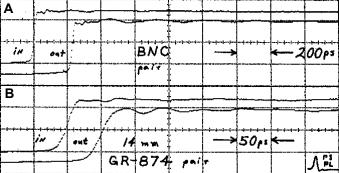
Figure 7: Step Response of BNC (top) and 14 mm, GR-874 (bottom) Connector Pairs
