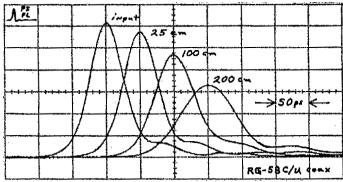
Figure 6: Impulse Response of Short Lengths of RG-58C/U
