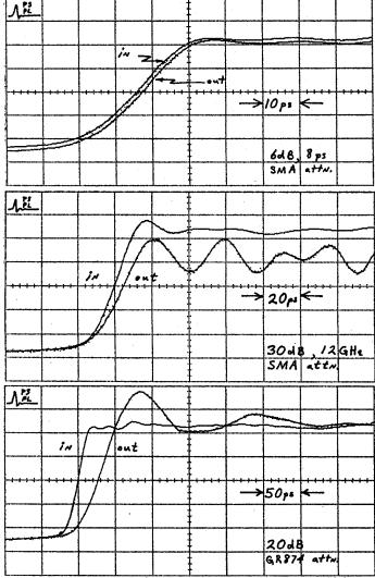
Figure 2: Examples of "Good" and "Bad" Attenuator Transient Response
