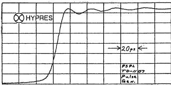
Figure 1: PSPL Model TD-1107 Pulse Generator Measured on HYPRESS Superconducting Sampling Oscilloscope
