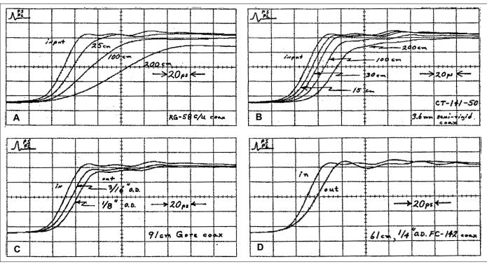
Figure 5: Transient Responses of Short Coaxial Cables
