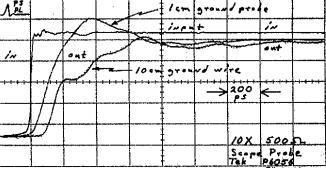
Figure 8: Step Responses of 10 X, 500 Ohm Signal Probes
