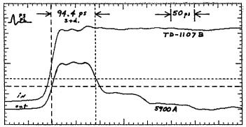
Figure 3: Time Base Calibration Using Short Circuit Stubs
