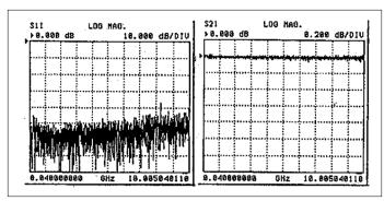
Figure 9: System Calibration Results for PSPL 100 Ohm Differential 10 GHz VNA
