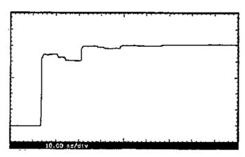
Figure 5: Pulse Step Response of two 5320A BALUNs Connected Back-to-Back. 10 ns/div.
