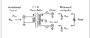
Figure 2: BALUN Transformer with Center-Tapped Output
