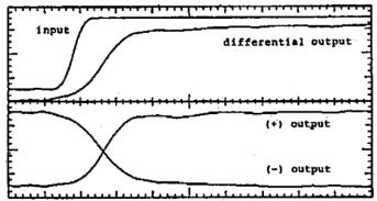
Figure 4: PSPL Model 5320A BALUN Pulse Response Input Step has 10 ps Risetime. Time Scale is 20 ps/div.
