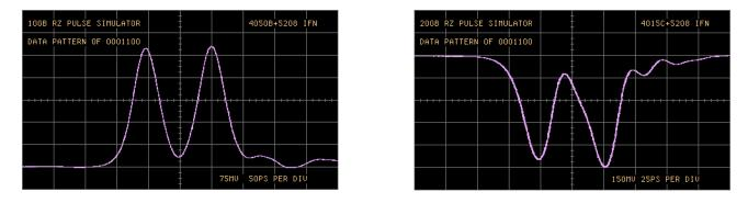
Figure 13: Simulated 10 and 20 Gb/s RZ pattern sequences of 0 0 0 1 1 0 0, using PSPL impulse generators
