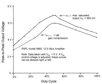
Figure 14: Amplifier max. output amplitude vs. input signal duty cycle
