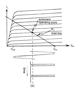
Figure 15: A Typical class A amplifier load line analysis
