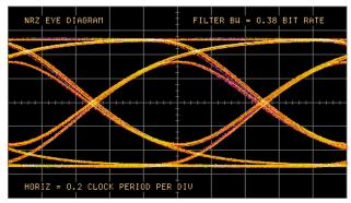
Figure 7: Limited bandwidth NRZ eye diagrams
