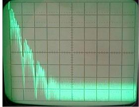
Filtered NRZ data, BW = 0.75 \* Bit Rate
