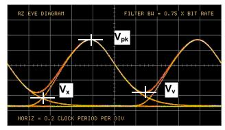
Figure 8: Limited bandwidth RZ eye diagrams
