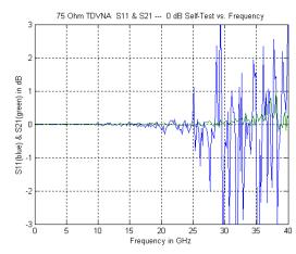
**Fig. 15** 75Ω TDVNA 0 dB self-test of repeatability and maximum frequency;  $S_{21}$  (green) and  $S_{11}$  (blue)
