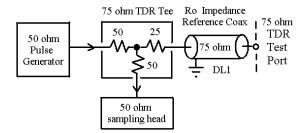
Fig. 9 Special 75  $\Omega$  TDR Tee for use in a 50  $\Omega$  system
