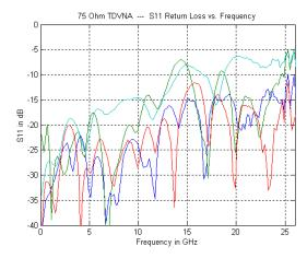
**Fig. 17** S<sub>11</sub> of 75Ω broadband coaxial components; DC Block (red), Bias Tee (green), 6 dB Tee (blue), and 25  $\Omega$  Series, 75 to 50  $\Omega$  Terminator (cyan).
