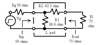
Fig. 2 Minimum Loss 50 / 75  $\Omega$  "L" Matching Pad
