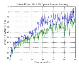
Fig. 14 75Ω TDVNA system self-test for dynamic range;  $S_{21}$  (green) and  $S_{11}$  (blue)
