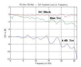
**Fig. 16**  $S_{21}$  of  $75\Omega$  broadband coaxial components; DC Block (red), Bias Tee (green), and 6 dB Tee (blue)
