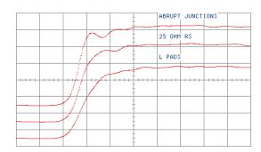
**Fig. 11** 75 Ω TDT test pulses with various Z matching networks, 100 mV/div and 20 ps/div
