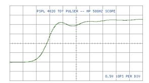
**Fig. 10** PSPL 4020 TDT pulser measured on HP 50 GHz oscilloscope, 0.5 V/div and 10 ps/div
