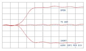
**Fig. 12** 75  $\Omega$  TDR — reflections from open, 75  $\Omega$ , and short; 60 mV/div & 20 ps/div
