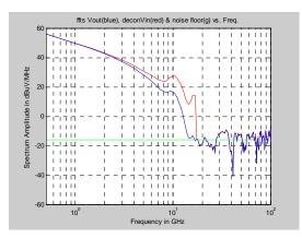
**Fig. 8** Frequency spectrum of Vout(f) (blue) and deconvolved Vin(f) (red)
