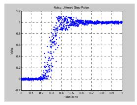
Fig 3 Distorted step pulse of Fig. 2, but with added vertical noise of 10 mV and 25 ps timing jitter
