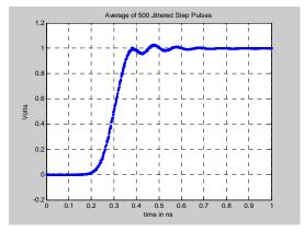
**Fig. 4** The result of signal averaging 500 noisy, jittery waveforms.
