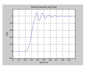
Fig. 2 Ideal test signal — a 1V, 100 ps rise Gaussian step with added overshoot and ringing
