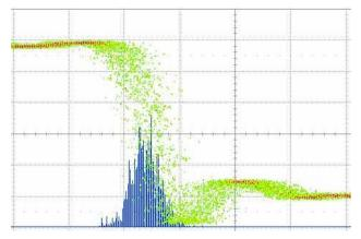
**Fig. 1** A pulse edge with Jitter. Blue trace is jitter histogram. 10 ps/div
