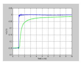
**Fig. 2** Pulse Response of Coaxial Cable. 20ps rise Input (blue) and Output (green) from 28 ft. of RG-58C/U.
