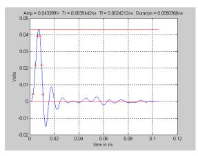
**Fig. 1** Step and Impulse Responses of PSPL/LeCroy SE-70, 70 GHz, 4.44 ps risetime, calibrated sampling head. PTB calibration [4] for 100 ps time window.
