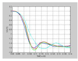
Fig. 5 Pulse response of PSPL attenuators. 8 ps falltime Input (blue), 5510V-10dB (green), 5510K-10dB (red) and 5510SMA-10dB (cyan). Attenuator waveforms scaled by 10dB for ease of comparison. Top plot 200 ps time window. Bottom plot 50 ps time window.
