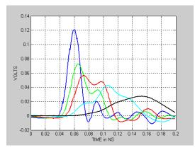
**Fig. 3** Step and Impulse Responses of RG-58C/U coaxial cables. Input 20ps Step or Impulse (blue), 9" (green), 1 ft. (red), 3 ft. (cyan) and 6 ft. (black) 200 ps time window.
