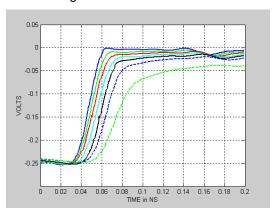
**Fig. 4** Step Response of Semi-Flex 0.141" SMA coaxial cables. 20 ps Step Input (blue), 6" (green), 12" (red), 18" (cyan), 1m (black), 4 ft (blue dash), and 8 ft (green dash). 200 ps time window.
