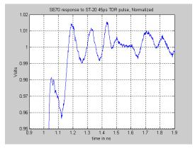
Fig. 3 SE-70's blow-by response to 45 ps TDR pulse. Settling time to 0 V topline expanded. 1%/div & 10 ns time window (top) & 1 ns (bottom). Ringing is generator artifact.
