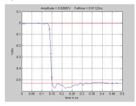
**Fig. 4** NPL calibration data for PSPL's gold standard, model 4015C pulse generator.  $T_{fall} = 11.2 \text{ ps.}$
