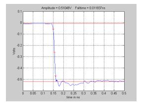
**Fig. 9** Deconvolved 4015 waveform.  $T_{fall} = 11.8 \text{ ps.}$
