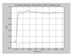
**Fig. 6** Comparison of normalized NPL data blue) and the 4015C waveform measured by the SE-70 sampler (red). Difference (green).
