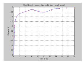
Fig. 7 Blow-By correction math model for Gold Std. SE-70 sampler. Blue trace is math model. Red crosses are measured blow-by data.
