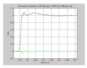
**Fig. 10** 4015C waveforms. Comparison of normalized NPL data (blue) and deconvolved SE-70 measurement (red). Difference (green).
