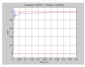
**Fig. 8** Gold Std. SE-70 step response including PTB calibration data and modeled Blow-by effects. 500 ps time window.  $T_{rise} = 4.75 \text{ ps}$ .
