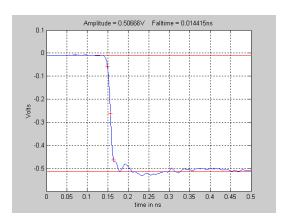
Fig. 5 SE-70 measurement of above NPL calibrated 4015C.  $T_{fall} = 14.2 \text{ ps.}$
