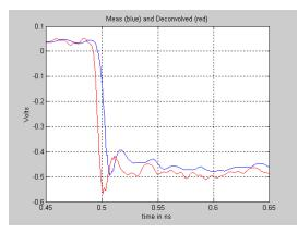
**Fig. 12** Deconvolution (red) of PSPL 4016 pulser. Measured waveform (blue), Deconvolved waveform (red), 5 ns (top), and 200 ps (bottom) time windows.
