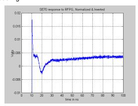
**Fig. 2** SE-70 blow-by response to RFPG, expanded vertical = 0.5% /div, 100 ns time window.
