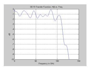
**Fig. 11** Frequency response of Gold Std. SE-70 sampling head.
