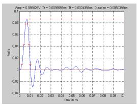
**Fig. 1** PTB step response (top) and impulse response (bottom) calibration data for PSPL's Gold Std. SE-70 sampling head. Step  $T_{rise} = 4.4$  ps & Impulse  $T_d = 5.0$  ps.
