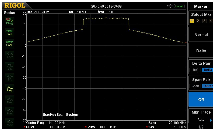
Fig. 16 Model 70-9B Amplifier output spectrum for max. drive level resulting in -12dB shoulders. P_{out} = +47.5\text{dBm} = 56\text{ watts rms} Totally unacceptable spectrum contamination.
