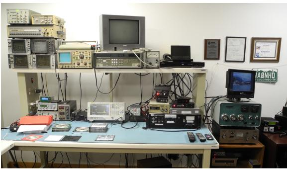
This is my electronics test bench. It contains a lot of analog TV test gear which I no longer use with DTV. The key test instrument is the Rigol spectrum analyzer.
