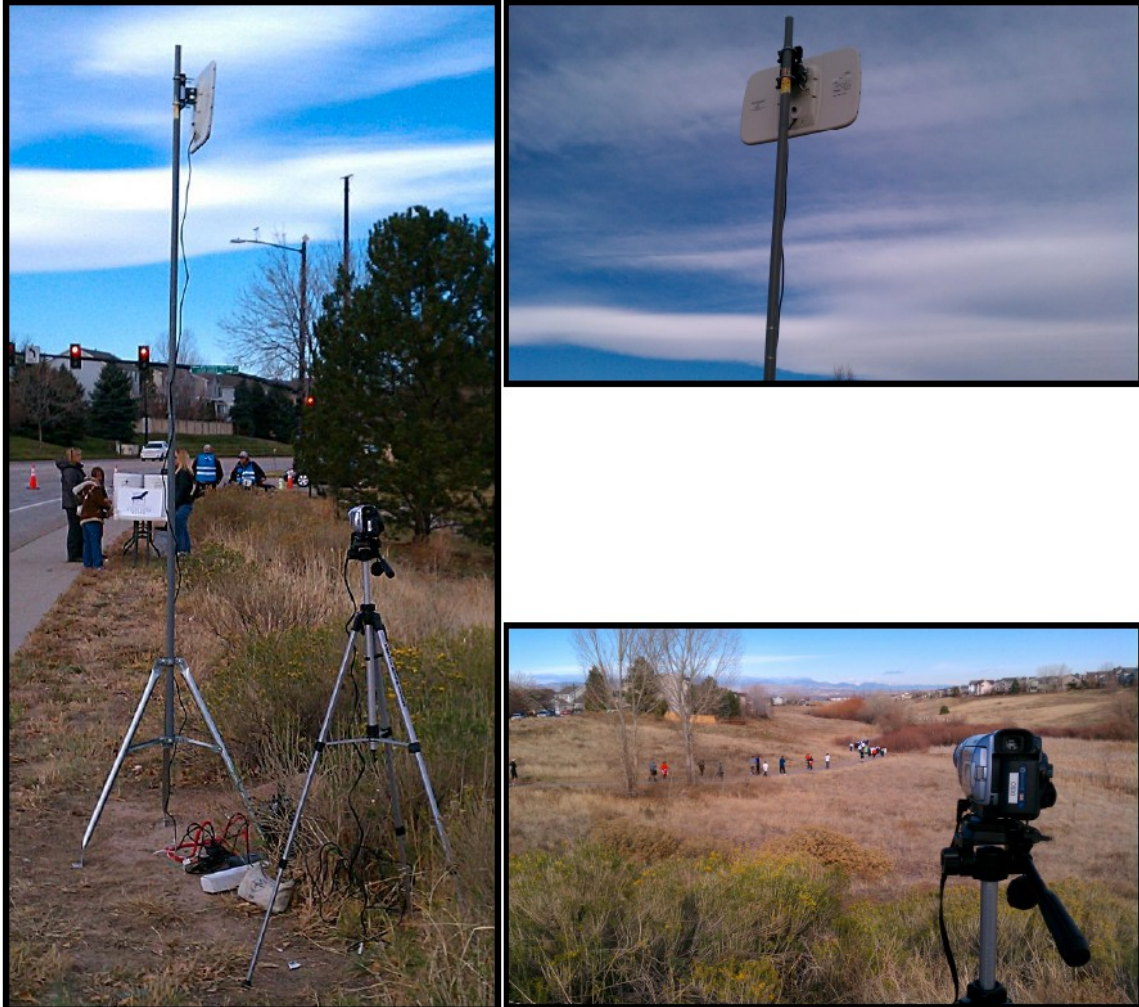
First year setup at the rest stop using a Ubiquiti PowerStation on a short mast and an analog NTSC camera that was converted to IP.
