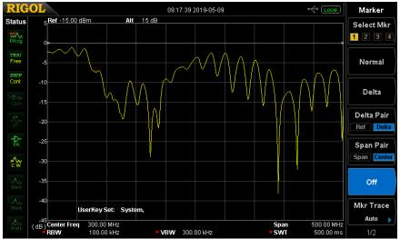
Return Loss of Comet CA-2X4SRN-NMO 2m/70cm mobile antenna. Sweep from 50 to 550 MHz, 50MHz/div & 5dB/div. Note: -14dB RL = 1.5:1 vswr, -10dB RL = 2:1 vswr & -6dB RL = 3:1 vswr
