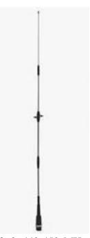
The Comet specs. for the antenna were: VSWR < 1.5:1 144-148 & 440-450 MHz, VSWR < 2:1 140-160 & 435-465MHz, Gain = 3.8dBi (2m) & 6.2dBi (70cm), 150 watts max., length = 40", NMO or PL-259 connectors available. The optional spring, model CA-SPR was ordered and installed in the antennas.
