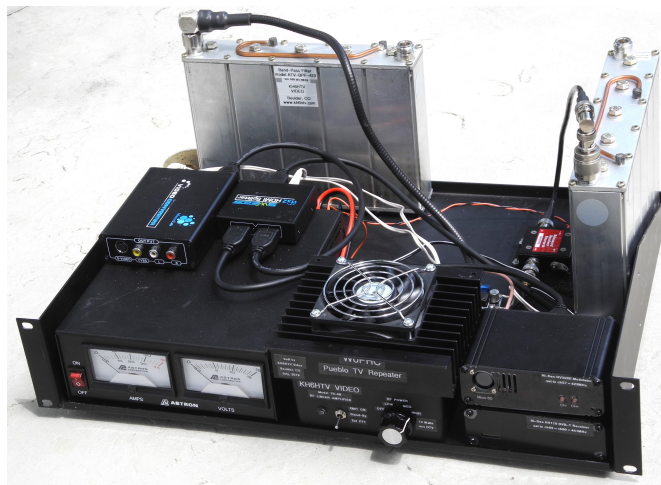
Fig. 1 A basic, 70cm, 10 Watt, DVB-T, Television Repeater
