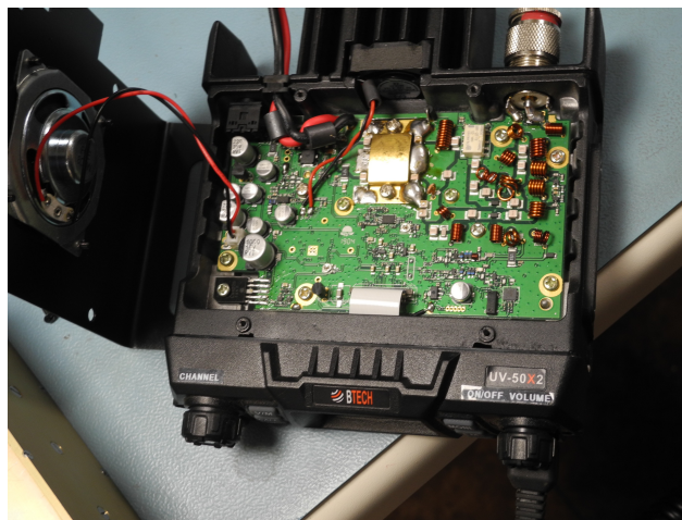
A peek inside the UV-50X2. This one has a blown final amp. No visual evidence of damage, but no RF out. Guess all the magic smoke got let out !
