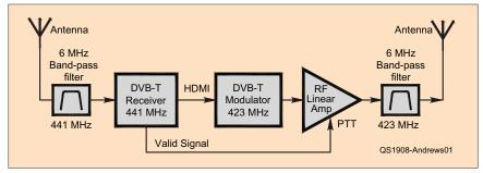
Figure 1 — Block diagram of a DVB-T repeater.
