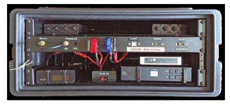
Figure 3 — A portable 70-centimeter DVB-T repeater built by KØDVB. [Matt Holiday, KØDVB, photo]
