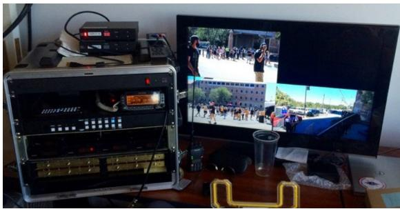
Fig. 2 The new BCARES Quad DVB-T Receiver and live, hi-definition images at a CU football game received on channels 57, 58 & 60. Note: ch. 59 is also possible.
