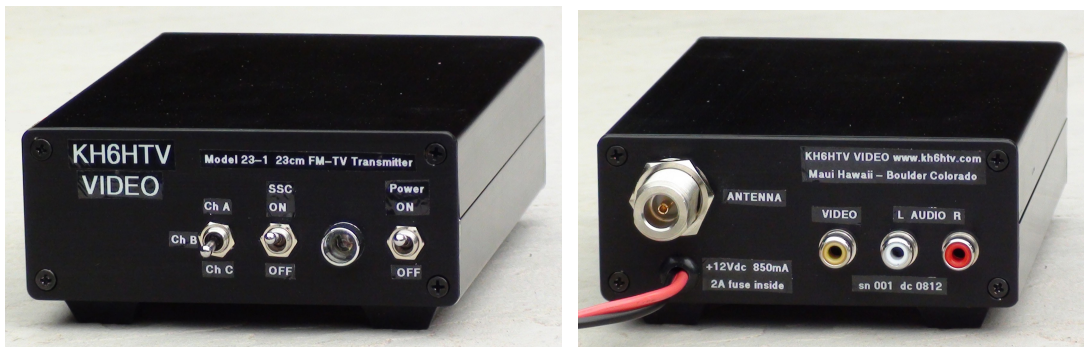
Fig. 8 KH6HTV Video model 23-8 FM-TV Modulator
