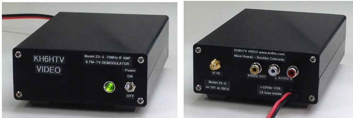
Fig. 11 KH6HTV Video Model 23-5, FM-TV Demodulator
