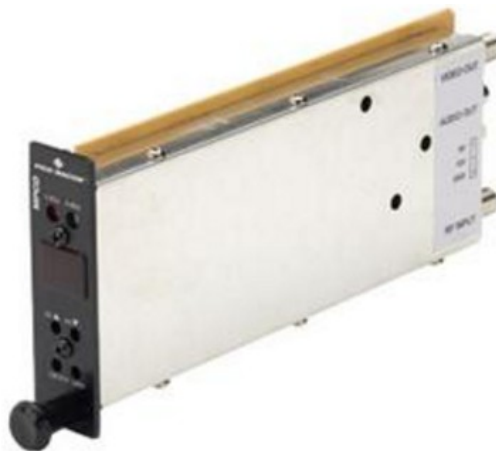
Fig. 10 Pico-Macom MPCD Demodulator
