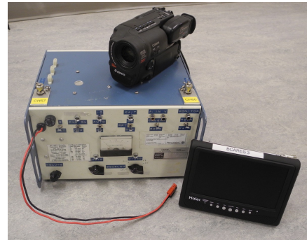
BCARES - Portable, 70cm, 10 Watt, ATV Repeater
