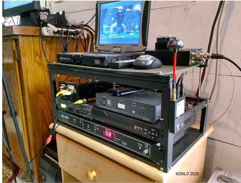
KD6ILO Mobile TV Transmitter Unit [70cm Analog] 8-input - XBand | Inputs 5cm, 23cm, IPTV & local cam | Rf Out: 10 watts
