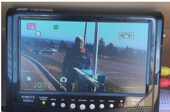
New 5.9GHz repeater transmitter as received 6 miles away on a rubber duck antenna.
