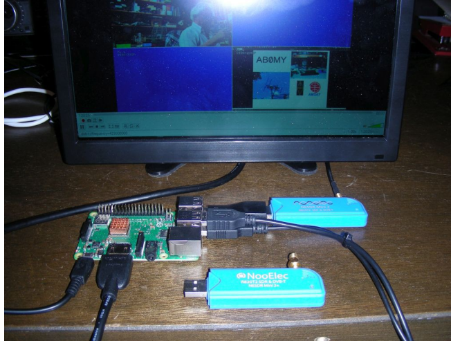
Live 70cm, DVB-T video image being received with RPi-3 using a Nooelec model NESDR Mini 2 SDR (spare in foreground.)
