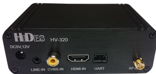
Hi-Des DVB-T modulator (left) &amp; set-top box receiver (right)
