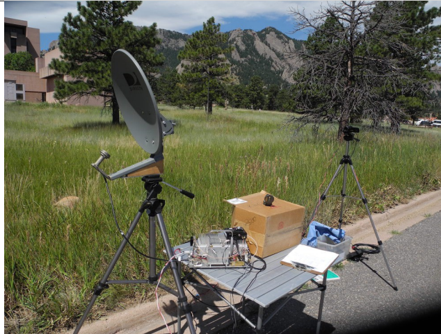
KH6HTV, 10 GHz, DVB-T setup at NCAR site
