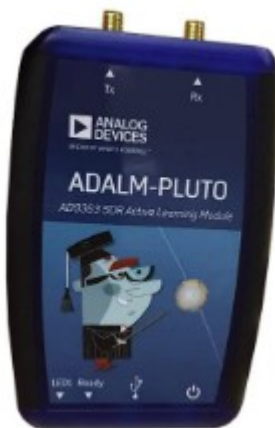
ADALM-Pluto (left) & Lime SDR Mini (right) --- DTV Transmitters
