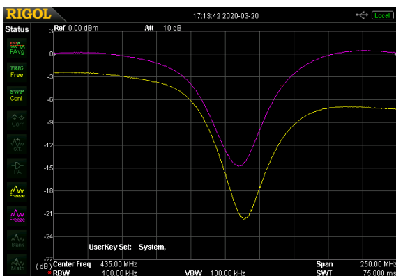
S21 Gain (left photo) & Return Loss (right photo) S11 = yellow trace, S22 = magenta trace center freq = 435 MHz, 250 MHz span, 3 dB/div & 25 MHz/div.
