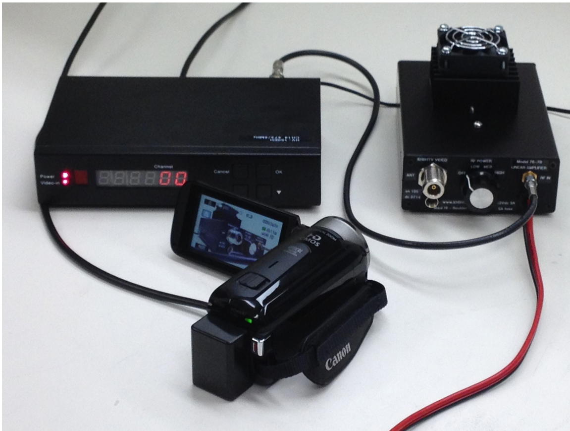
Fig. 6 A typical amateur DVB-T transmitter consisting of a camcorder, DVB-T modulator and an RF power amplifier. Shown is a Canon camcorder, Hi-Des model HV-100EH modulator and a KH6HTV Video model 70-7B amplifier.
