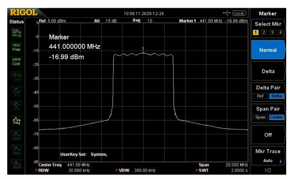
This photo shows the proper setup for measuring a DVB-T signal. The signal was direct from a Hi-Des HV-320E modulator set for 441 MHz, 6 MHz bandwidth and QPSK. The RMS power of this signal was +5.3dBm as measured with the HP-432A power meter.
