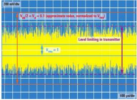
oscilloscope display of DVB-T signal - R&S
