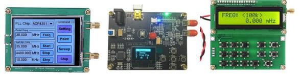
Fig. 2 Three versions of a Chinese, ADF-4351, Frequency Synthesizer board
