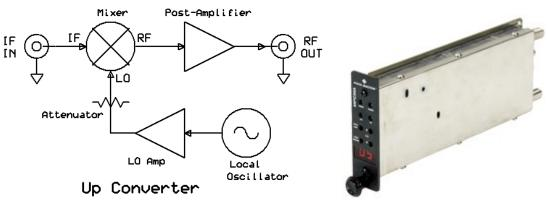
Fig. 7 Block Diagram for an Up-Converter Fig. 8 CATV analog VUSB-TV modulator
