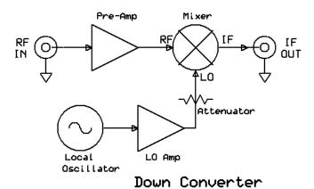
Fig. 1 Block Diagram for a microwave down converter.
