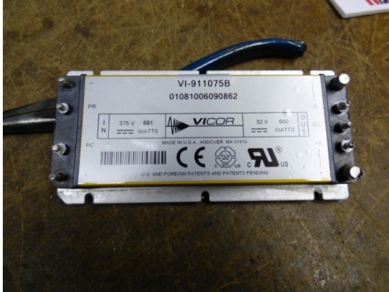
Power supply, 375VDC in 32VDC out @ 18 A max.
