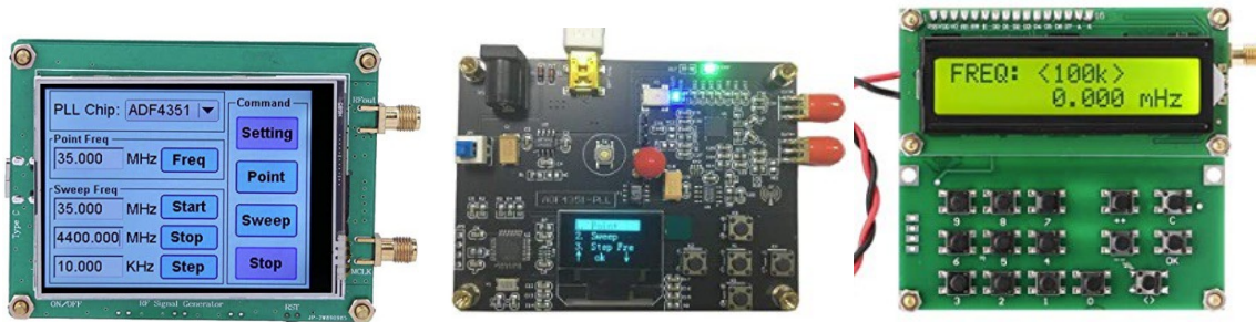
Fig. 2 Three versions of a Chinese, ADF-4351, Frequency Synthesizer board
