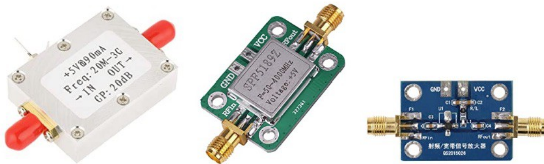
Fig. 4 Typical, low cost, amplifier modules from China
