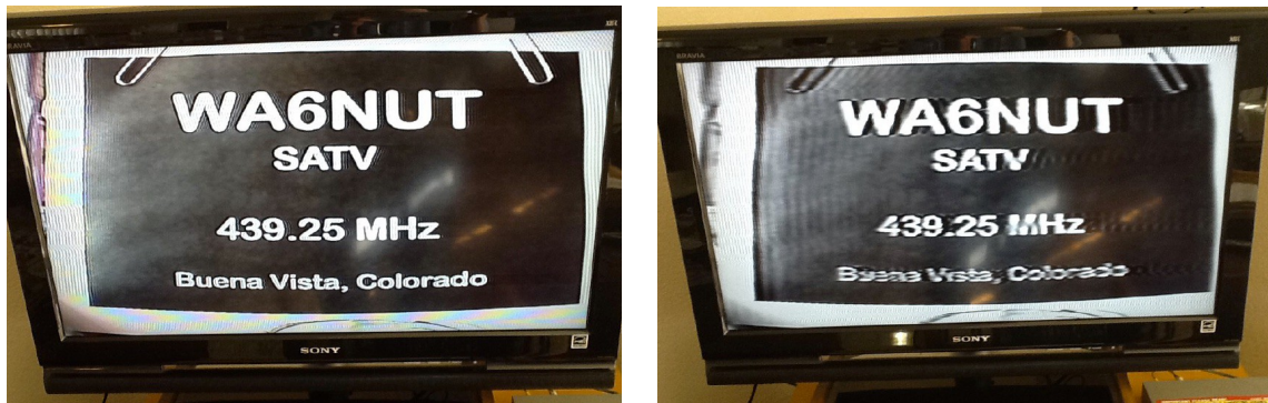
Fig. 3 The received ATV image, without the low pass video filter (on the left) and with the 1 MHz low pass (on the right). Note the distortion in the QTH ID and lack of color in the received SATV image.
