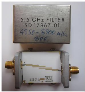
I have soldered a piece of hookup wire to the SMA connector as a attempt to repair the filter. The IL is down quite a bit and so the filter has been set aside to be attended to later. I hope to possibly recover some of its band pass capabilities.
