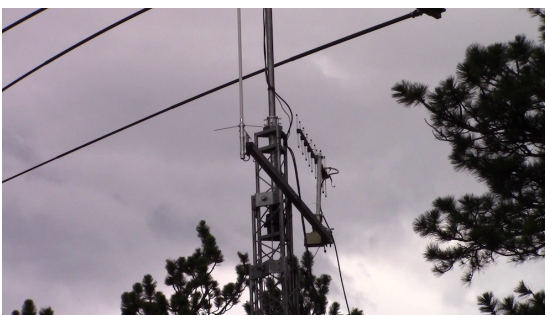
The 70cm Yagi used for TV link
