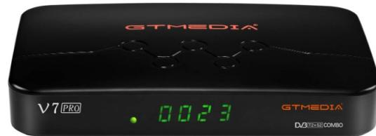
**KH6HTV VIDEO** offers for sale a consumer grade, digital TV receiver which we have pre-programmed for operation on the amateur **70 & 33cm** bands (420-450 MHz & 902-928 MHz). It has been programmed to receive, eight, 6 MHz ATV channels for DVB-T.
