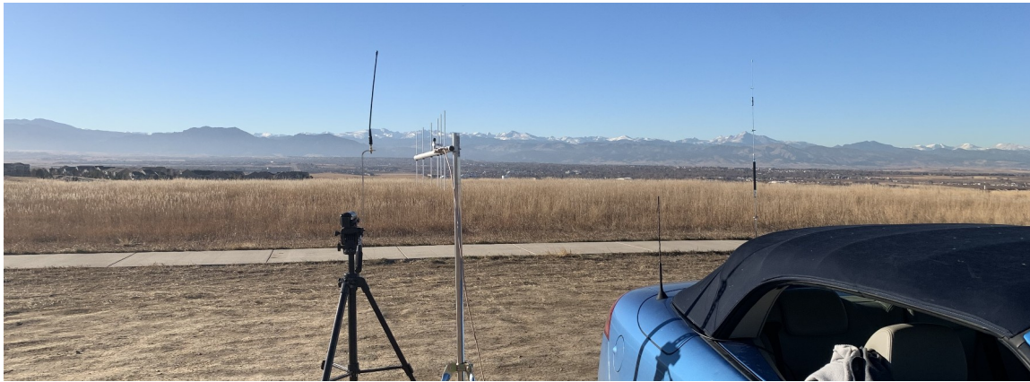
View from Lowell Blvd. test site towards W0BTV repeater The line-of-sight distance to the repeater was about 13 miles. The repeater's rf signal level to our reference antenna was about -71dBm.
