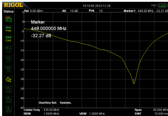
Diamond X50NA, Base Station Omni >14dB (436-453), >10dB (426-455)
