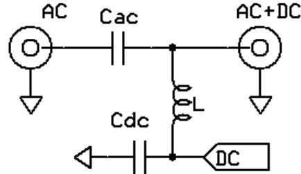
A Bias Tee is used to either insert or extract DC power to / from a coaxial cable. It can be used to send dc power up a cable to an antenna mounted pre-amp or coax relay. The Model BT-UHFa has a useful frequency response covering from 2m to 23cm bands (144 MHz to 1.3 GHz). It is rated to 50 Vdc and 2 Amps.
