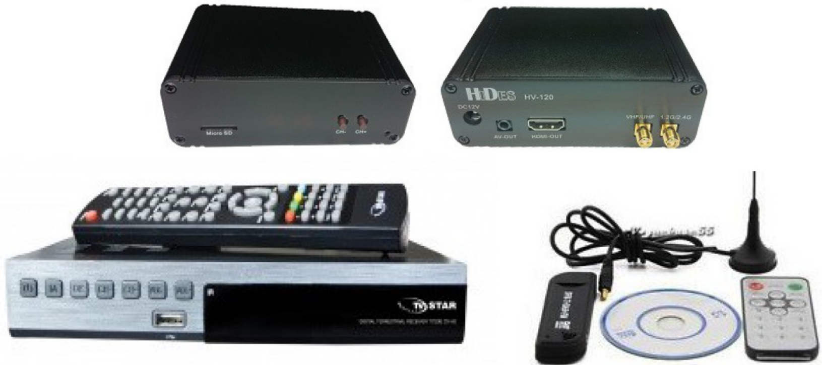
Fig. 15 Set-Top box receivers for DATV & USB dongle TV tuner
