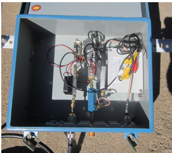
Fig. 28 5.9GHz, FM-TV Transmitter enclosure & antenna -- roof top mounted.
