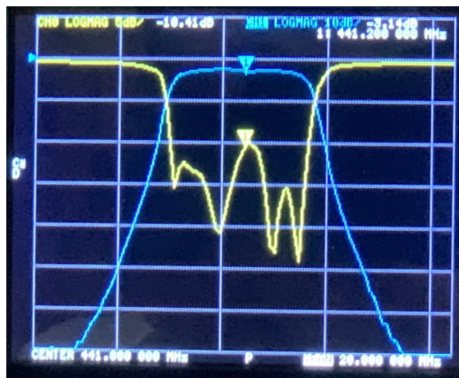
Fig. 20 Channel 60, 70 cm, 7 pole, inter-digital, Band-Pass Filter built by Don, N0YE. Used as the front end for the 70 cm receivers. S21 (blue) at 10dB/div. S11 (yellow) at 5dB/div. Center Freq. = 441 MHz, Span = 20 MHz. Measured with NanoVNA.
