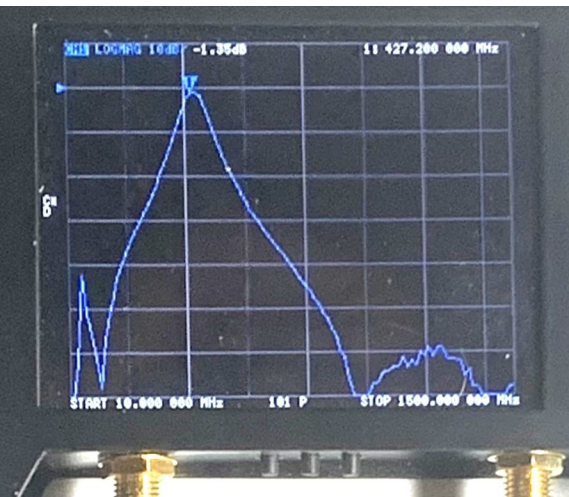
S21 Gain sweep from 0 to 1.5GHz, 10dB/div
