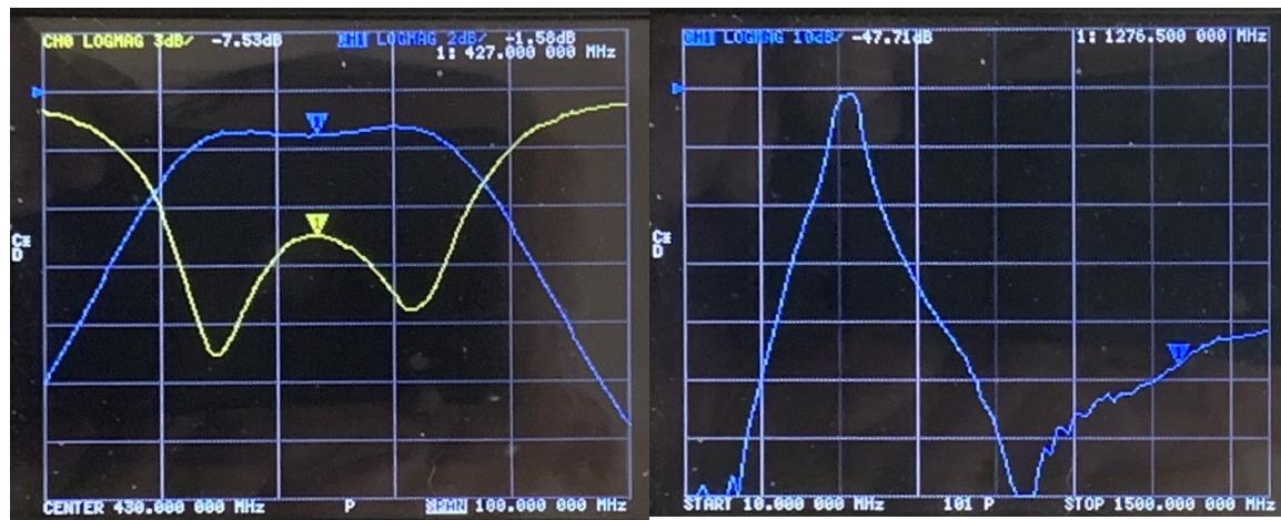
430 MHz center freq., 100 MHz span
