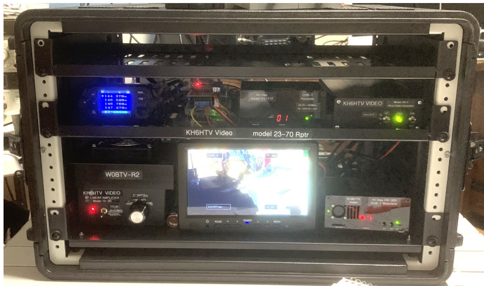
Fig. 1 This photo shows a 70cm in-band repeater built for BCARES. All the components were assembled onto three 1U, 19", relay rack shelves. This proto-type used the 70-9B, 10 Watt, rf power amplifier. It also included a 2m FM receiver, ABOMY - Arduino DTMF decoder / relay, video monitor and +13.8Vdc power supply.
