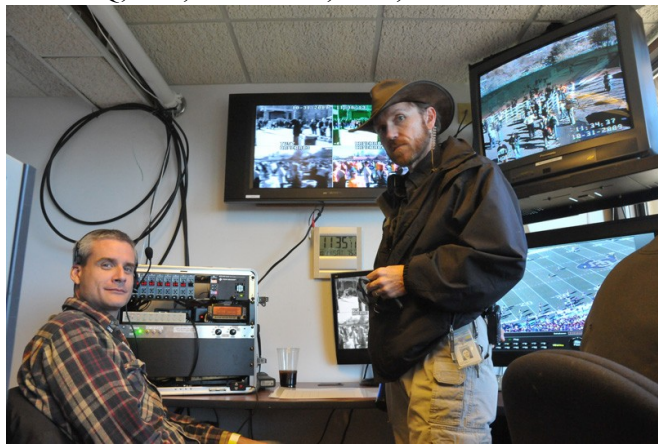
Fig. 34 Dave, K10HG & Mark, KB0LRS, BCARES TV net control in the CU police chief's command post receiving four simultaneous, TV signals on channels 57-60 (70cm), from BCARES portable TV cameras/transmitters.
