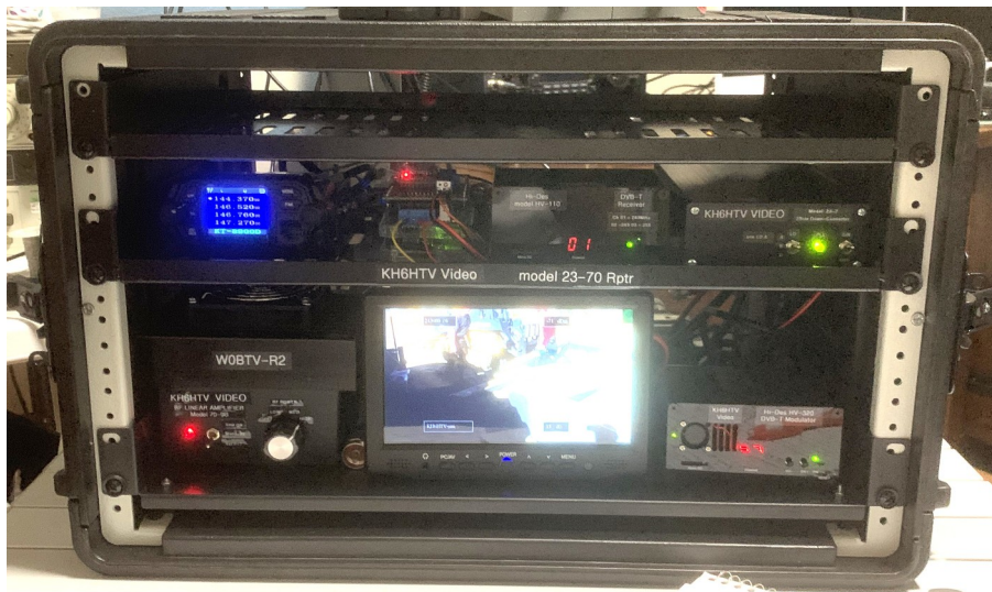
Fig. 29 A basic, 70 cm, 10 Watt, DVB-T, Television Repeater
