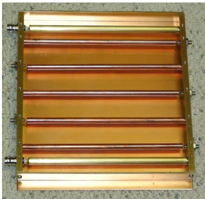
Fig. 21 A 70 cm, 6 MHz bandwidth, inter-digital, band-pass filter. Shown with the top cover removed. S21 frequency response 10dB/div & 5MHz/div
