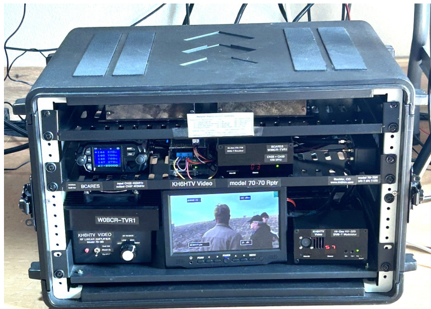
Fig. 1 This photo shows a 70cm in-band repeater built for BCARES. model 70-70R, s/n 1. All the components were assembled onto three 1U, 19", relay rack shelves. This proto-type used the 70-9B, 10 Watt, rf power amplifier. It also included a 2m FM receiver, ABOMY - Arduino DTMF decoder / relay, video monitor and +13.8Vdc power supply.
