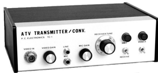
Fig. 1 Tom, W6ORG, and his model TC-1 70cm AM-TV Transmitter introduced at Dayton in 1977. The "work-horse" of ATV for many years.
